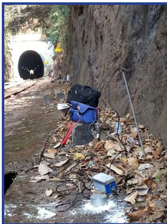
Photo 9: View of vibration monitoring outside downline tunnel portal and along the tunnel alignment
