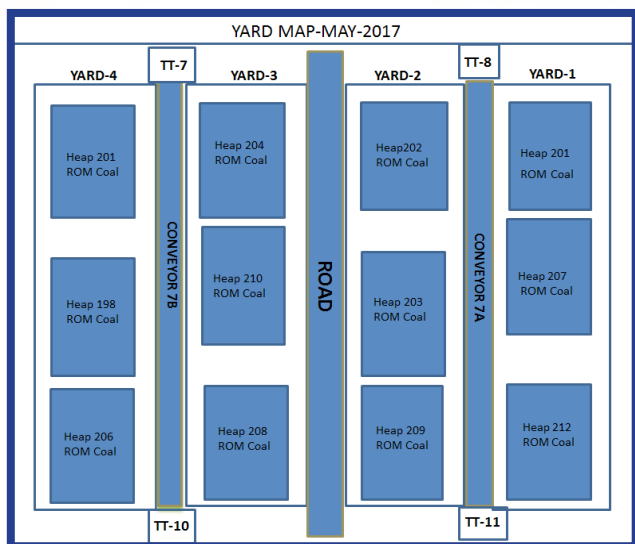
Fig 1 : Representation of Layout of coal yards
