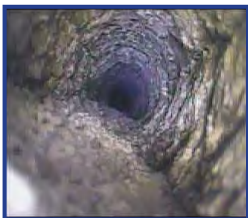
(a) With controlled blasting (no damage)
