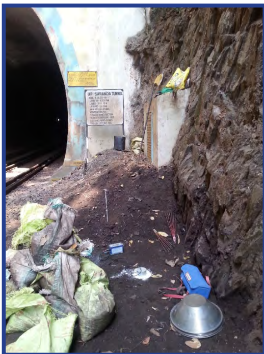
Photo 9: View of vibration monitoring outside downline tunnel portal and along the tunnel alignment
