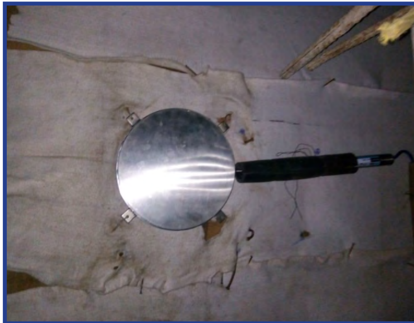
Fig 3: CPC attached inbye of barricade.
