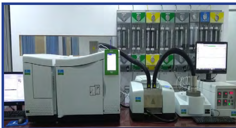
STA-8000 with off line and online FTIR and GC-MS (PerkinElmer)
