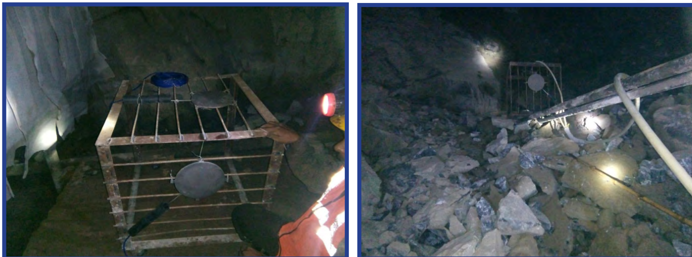
Fig 4: TPC installation inside the stope.
