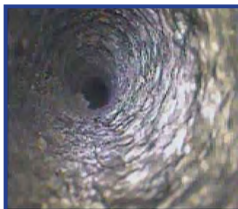
(b) With conventional blasting (damage)
